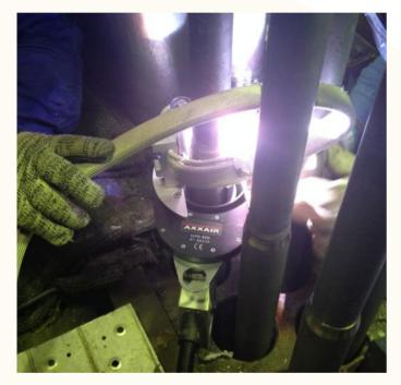
This type of machine can be used to weld carbon steel tubes.
