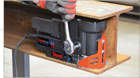
Compact design for height restricted areas. Detachable feed lever can be fixed from either side
