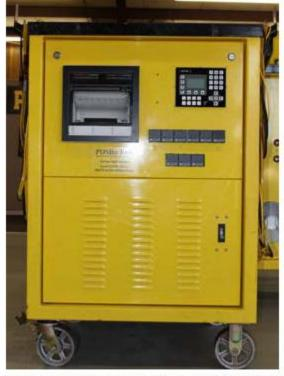
\* Note: This Machine is Capable of Operating (27) 80V Ceramic Pad Heaters Simultaneously when Stress Relieving.
