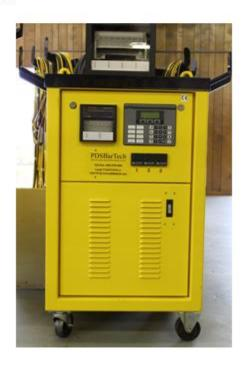
\* Note: This Machine is Capable of Operating (9) 80V Ceramic Pad Heaters Simultaneously when Stress Relieving.
