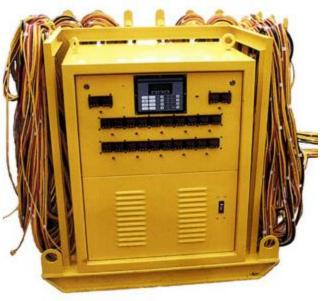
\* Note: This Machine is Capable of Operating (36) 80V Ceramic Pad Heaters Simultaneously when Stress Relieving.
