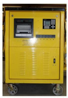
\* Note: This Machine is Capable of Operating (18) 80V Ceramic Pad Heaters Simultaneously when Stress Relieving.
