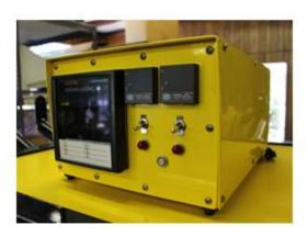
\* Note: This Machine is Capable of Operating (6) 80V Ceramic Pad Heaters Simultaneously when Stress Relieving. Requires at least a 300A Welding Machine as a Power Source.
